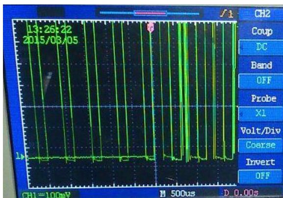
Figure 7: Waveform for RF transmitter
